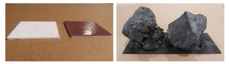
These photographs shows the samples before exposure and the comparison after 10 mins at 600°C.
